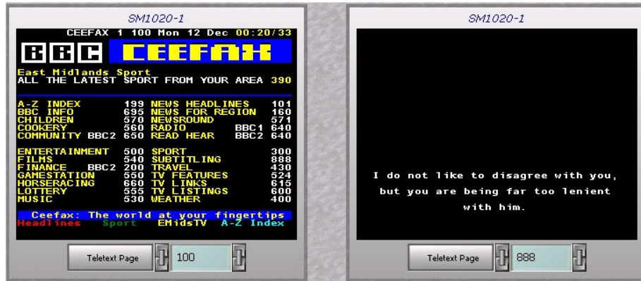
Modules showing recorded and decoded VBI data e.g. Tele-text and subtitle caption pages
